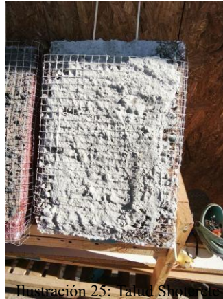
Figura 4.8 Caja minera Shotcrete Normal.
